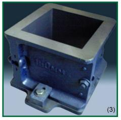
Cube moulds are usually 150mm x 150mm x 15 mm (or 100mm x100mm x100mm) and can be made from steel or polyurethane. The cube moulds must be manufactured to the specifications / standards of the relevant body, in the UK it is the British Standards Institute to this specification BS EN 12390-1:2000.
